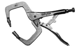
CORNER ALIGNMENT TOOL Modified vice grip can facilitate installation of corner clips.
